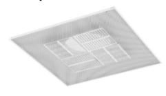
Titus perforated ceiling diffusers are designed for both heating and cooling applications. A tight, uniform, horizontal blanket of air protects the ceiling against smudging. Discharge pattern is easily adjusted by unlatching and dropping the perforated face, then rotating the pattern controllers.
