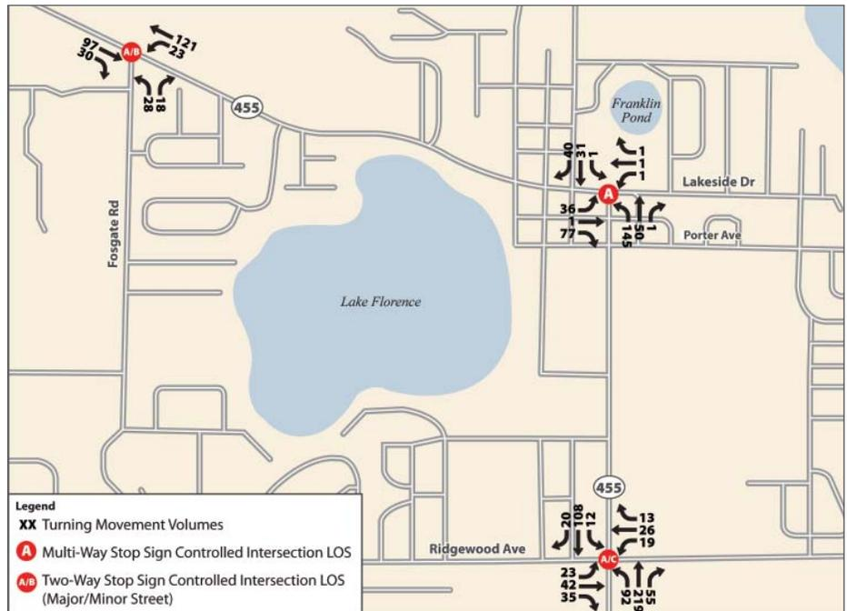
Figure 14 - Existing PM Peak Hour Turning Movement Volumes and Intersection LOS
