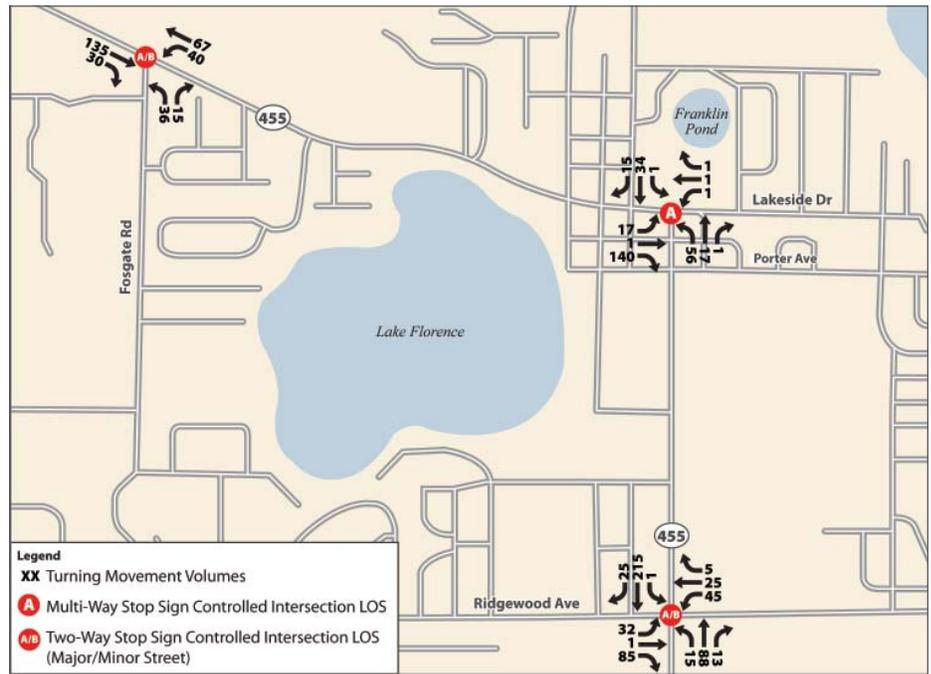
Figure 13 - Existing AM Peak Hour Turning Movement Volumes and Intersection LOS
