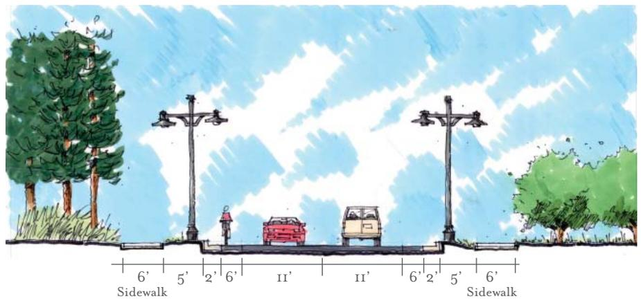
Figure 36: Curb and Gutter Section
