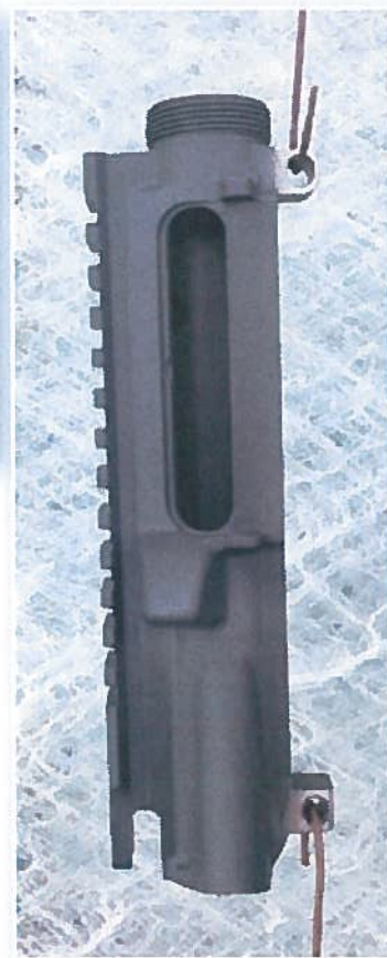
A sufficiently blasted anodized part.
