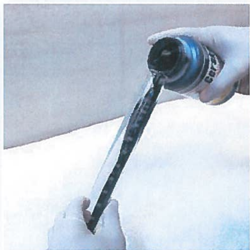
1.) Pour the desired quantity of Cerakote into a glass graduated cylinder.
