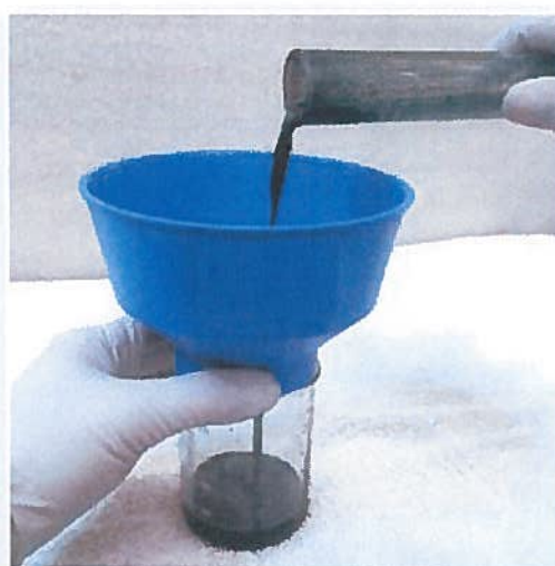
4.) Pour mixed coating through a 100 mesh strainer for all H or C-Series products, as shown (NIC Part # SE-139).
